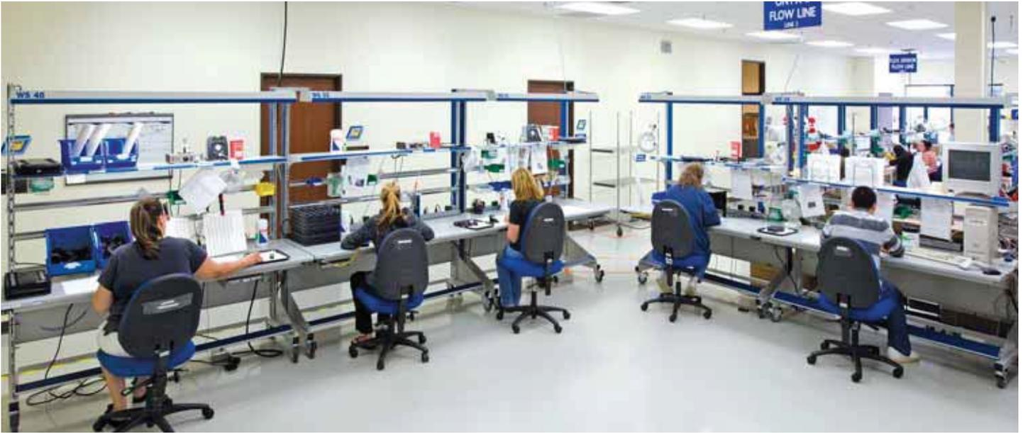
*Workcells for assembling pulse oximeters take advantage of the flexible configurability of the Arlink® 8000 system. Whether the task is progressive assembly or piece work, mobile Arlink 8000 workstations can be quickly and easily configured to accommodate workflow.*
