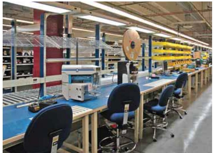
*Technical electronic workstations have the versatility to adapt to a wide range of tasks. At this manufacturing facility for electric power systems, tech legs are combined with the VSI accessory system and integrated with a conveyor system for maximum productivity on the assembly line.*
