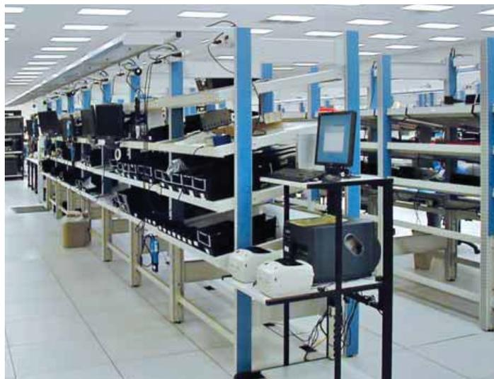
Flow racks can be used to stage and deliver parts utilizing gravity, reducing material handling time and costs. Bins or totes are loaded on flow rack frames from the rear, and as operators remove one from the front, a new bin glides forward on rollers. Similarly, flow rack frames can be inclined away from an operator to allow removal of completed work.
