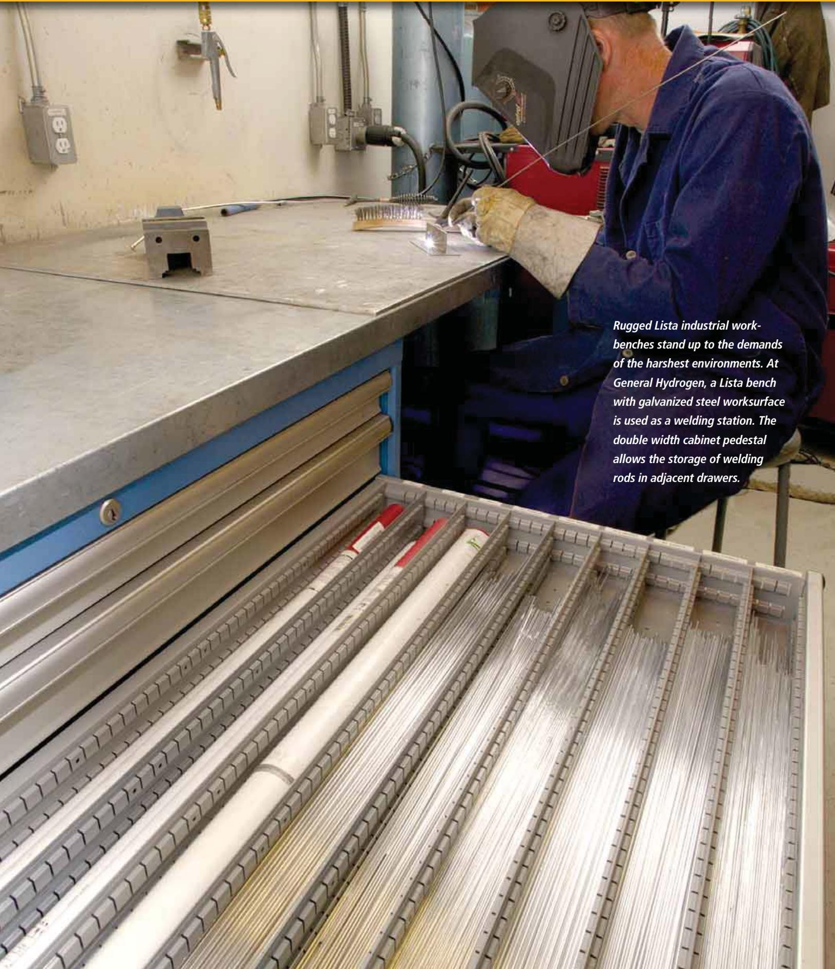
*Rugged Lista industrial workbenches stand up to the demands of the harshest environments. At General Hydrogen, a Lista bench with galvanized steel worksurface is used as a welding station. The double width cabinet pedestal allows the storage of welding rods in adjacent drawers.*
