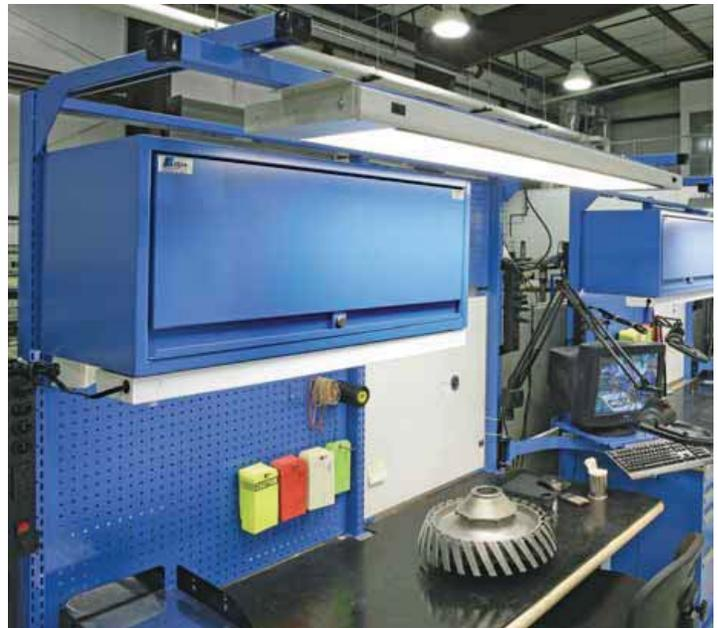
Articulating arms allow free and simple repositioning of a wide range of Nexus System accessories. Arm swings 180° for easy ergonomic access, and has a 75 lb. capacity. All accessories include arm and mounting bracket.
