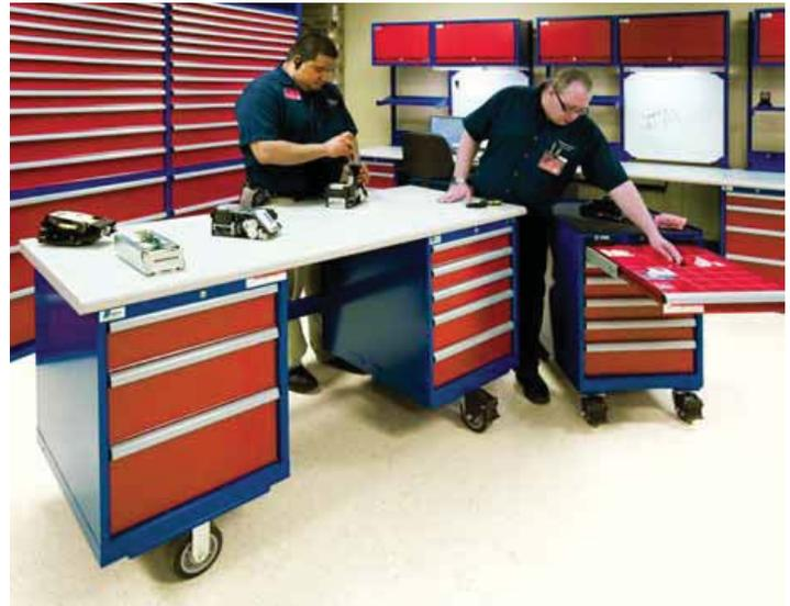
*The mobile workbench used at this electronic repair facility brings repair tools and parts right to the point of use, without sacrificing durability and drawer storage space. The companion mobile storage cabinet (designed to be stored between the workbench cabinet pedestals) adds to the flexibility of this arrangement. For information on ordering mobile workbenches with two cabinet pedestals, contact your Lista distributor.*
