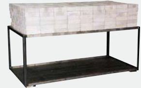
Brick Static Load Test
