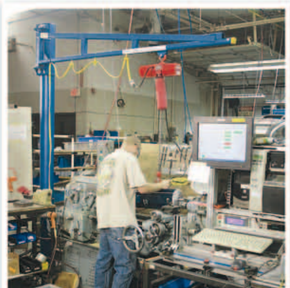
Floor Mounted TSJ150 in motor assembly area with light duty chain hoist
