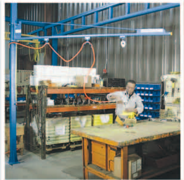
Floor Mounted TSJ50 with nut runner in refurbishing bay
