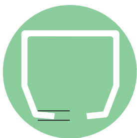
2-degree taper keeps the trolley centered
