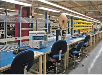
Technical electronic workstations have the versatility to adapt to a wide range of tasks. At this manufacturing facility for electric power systems, tech legs are combined with the VSI accessory system and integrated with a conveyor system for maximum productivity on the assembly line.
