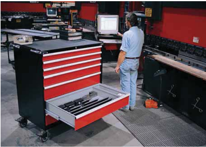
Mobile cabinets bring tooling to work areas in manufacturing settings.
